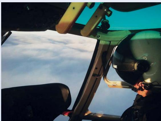
4 The autopilot is engaged, giving our pilot a moment to complete all IFR checks. As long as we're above the clouds, it's beautiful and sunny. But we'll have to come down through the clouds to land. The autopilot is programmed for our descent and the control tower in Kalamazoo follows us on radar as we approach their runway.
